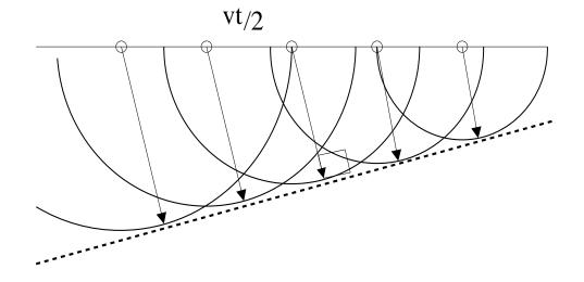
Reflecting surface must be tangent to each wavefront circle - envelope of circles.
