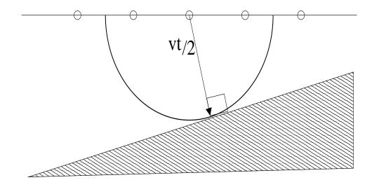
Reflection occurs at the place and time at which the wavefront is *tangent* to the reflecting surface - the *specular* (mirrorlike) reflection principle. Radius from source/receiver point is *normal* (perpindicular) to surface.
