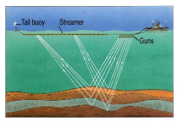
*Multiple Offsets* = data that's actually measured. Can either *fake* ZO data from multioffset data (1970's technology) or directly use MO data - routine today.
