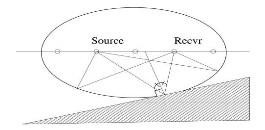
Reflection occurs at the place and time t at which ellipse with focii at source, recvr, diam = vt is *tangent* to the reflecting surface - the *specular* (mirrorlike) reflection principle. Bisector of lines from source and receiver points is *normal* (perpindicular) to surface (*Snell's law*)  $\Rightarrow$  surface is *envelope* of ellipses.
