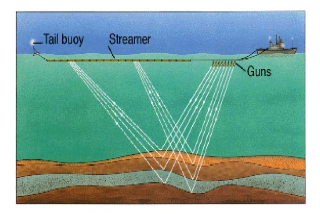
*Offset* = distance from source to receiver. Picture shows "near" and "far" offsets.
