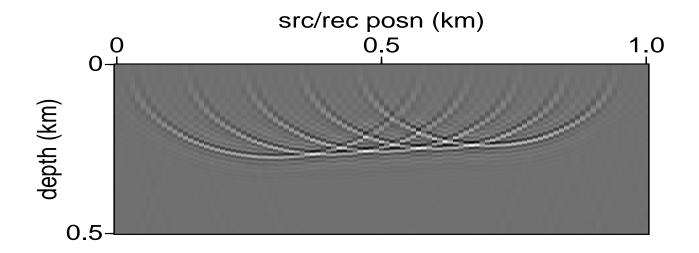
(2) then sum the resulting images, one for each source/receiver point (this figure shows 5 of the 101 source/receiver images added up, at 0.3, 0.4, 0.5, 0.6, 0.7 km from left edge).
