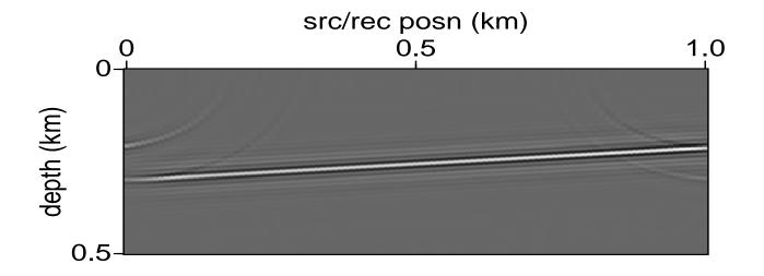
(2) then sum the resulting images, one for each source/receiver point (this figure shows all 101 source/receiver images added up - the wavefront envelope is recovered, sitting exactly on the reflecting surface!)
