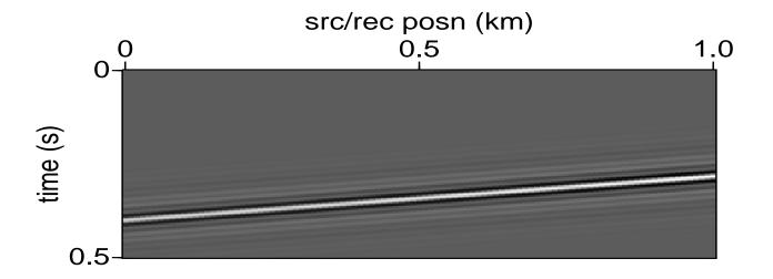
Zero offset simulated data for reflecting surface at depth z = 0.3 km at left edge (x = 0 km), sloping upwards to the right at 5 deg. 101 source/receiver points, spaced 10 m apart, from left to right.
