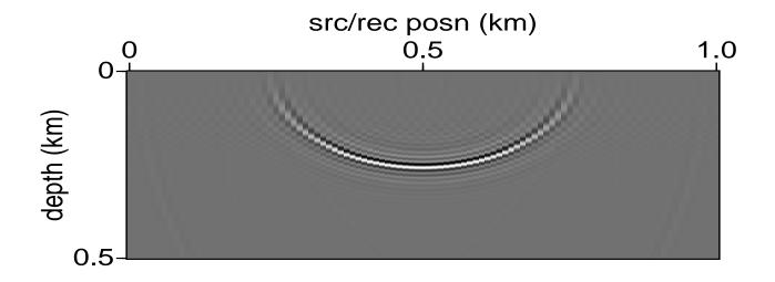
(1) for each source/receiver point each sample time t (usually multiples of 2 ms or 4 ms), *place* the sample value at all possible image points at distance vt/2 (circle).
