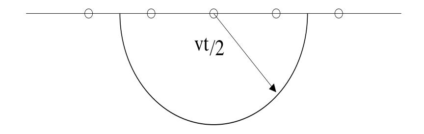
v = sound speed (or *velocity*) - 330 m/s in air, 1500 m/s in water, 2000 - 5000 m/s in sedimentary rock.
