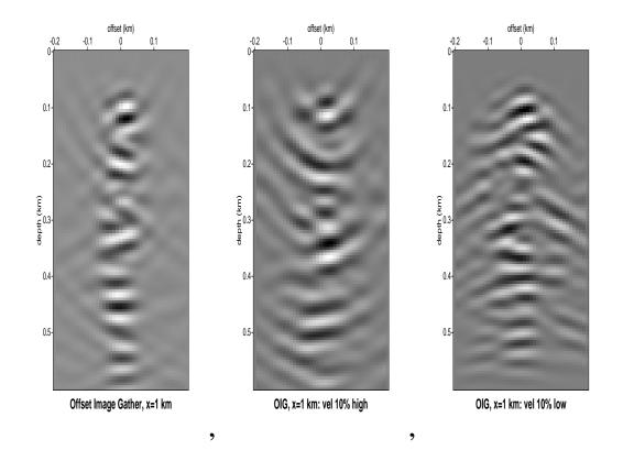
Two way reverse time horizontal offset S-G image gathers of data from random reflectivity, constant velocity. From left to right: correct velocity, 10% high, 10% low.
