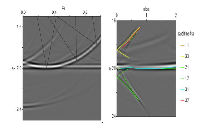
**Left:** Const. *h* slice of  $\overline{G}d$ : several refl. points corresponding to same singularity in  $d^{\text{obs}}$ . **Right:** CIG (const. *x*, *y* slice) of  $\overline{G}d$ : not smooth in *h*!
