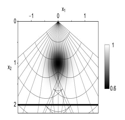
Example (Stolk & WWS, 2001): Gaussian lens over flat reflector at depth z ( $r(\mathbf{x}) = \delta(x_1 - z)$ ,  $x_1 = \text{depth}$ ).
