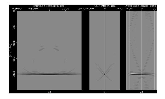
Lens data, shot-geophone migration [B. Biondi, 2002] Left: Image via DSR. Middle:  $\overline{G}[v]d$  - well-focused (at h = 0), i.e. in range of  $\chi$  to extent possible. Right: Angle CIG.
