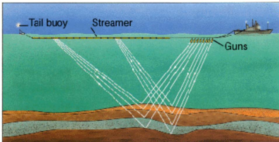
Airguns = **source** of sound. Streamer consists of hydrophone **receiver** groups. Each group records a **trace** (time series of pressure) for each **shot** = excitation of source. Source-receiver distance = **offset**.
