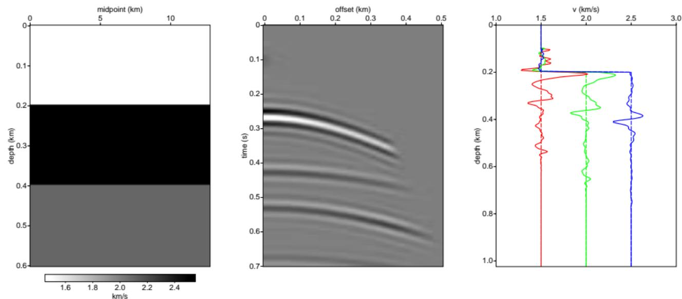
Left: Layered model. Middle: response to point source in center, 4-10-30-40 Hz bandpass wavelet. Right: OLS inversions, dashed=initial, solid=final. Quasi-Newton iteration terminated when gradient reduced by  $10^{-2}$ .
