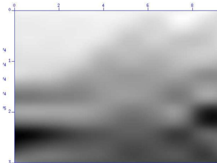
Starting velocity model for waveform tomography. Data: Born version of Marmousi, fixed receiver spread across surface.
