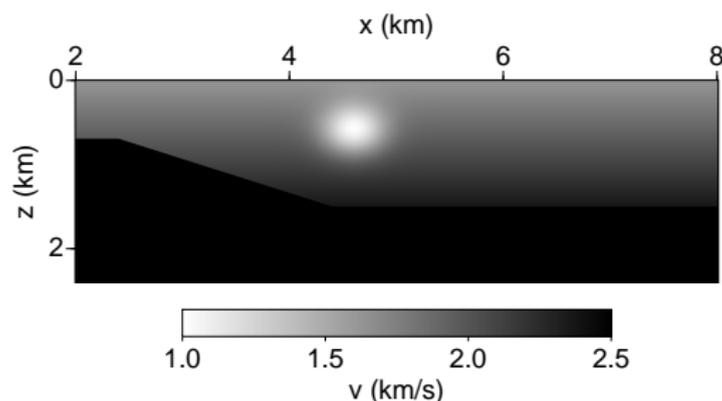
Velocity model after Valhall field, North Sea. Note sloping reflector at left, large low-velocity lens (modeling gas accumulation) in center. Both tend to produce multipathing. (Thanks: M. de Hoop, A. Malcolm)
