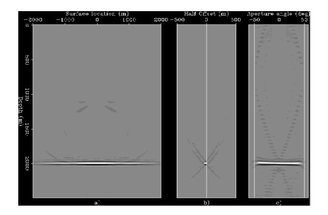
S-G migration of lens data. Left: image (h = 0 section) Center: CIG at x = 1.0km Right: Angle CIG (Radon of CIG in h, z) [Thanks: Biondo Biondi]
