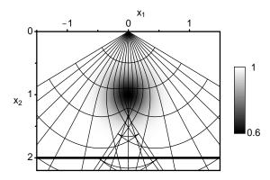
Example: Gaussian lens over flat reflector at depth z ( $r(x) = \delta(x_1 - z)$ ,  $x_1 = depth$ ).
