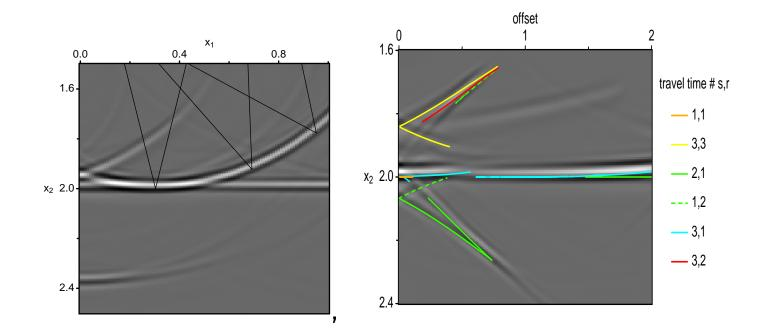
Common offset migration of lens data. Left: image at offset h = 0.3 km Right: CIG at x = 1.0 km - not smooth in h!
