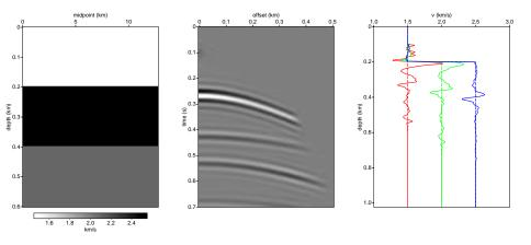
Left: Layered model. Middle: response to point source in center, 4-10-30-40 Hz bandpass wavelet. Right: LS inversions, dashed=initial, solid=final. Quasi-Newton iteration terminated when gradient reduced by  $10^{-2}$ .
