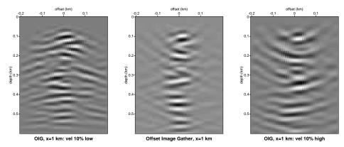
RTM space shift image gathers  $(I_D(\mathbf{x}, \mathbf{h}))$  from velo model  $v + \delta v$ , v = const.,  $\delta v =$  randomly distributed point diffractors. Left to Right: migration velocity = 90%, 100%, 110% of true velocity.
