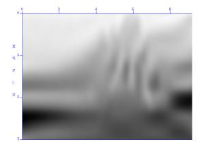
Final velocity (47 iterations of descent method). Note appearance of high velocity fault blocks.
