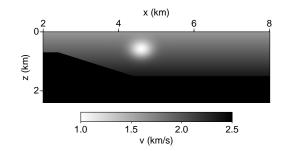
Velocity model after Valhall field, North Sea. Note sloping reflector at left, large low-velocity lens (modeling gas accumulation) in center. Both tend to produce multipathing. (Thanks: M. de Hoop, A. Malcolm)
